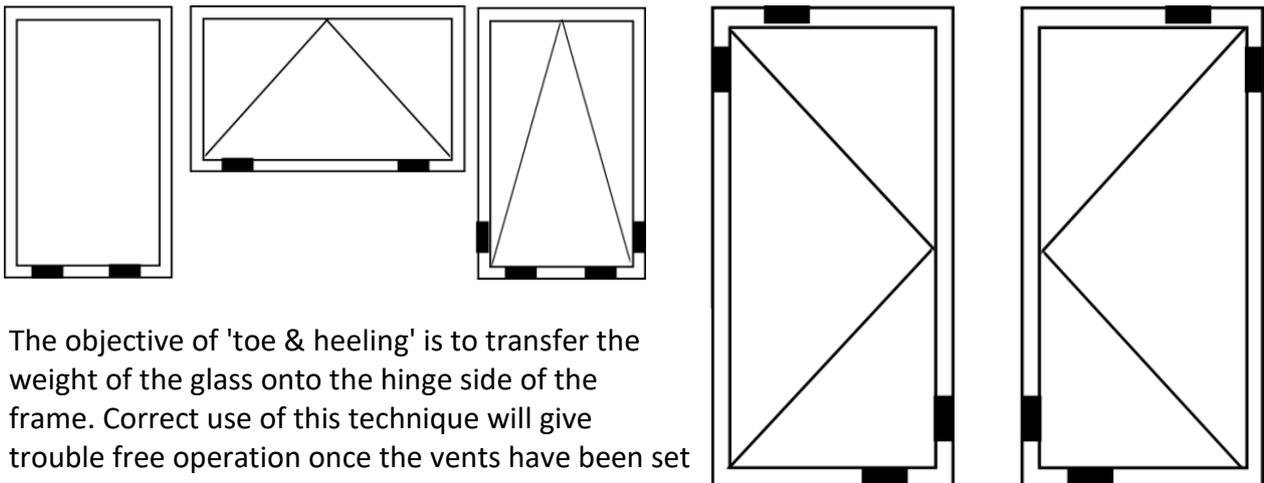
The objective of 'toe & heeling' is to transfer the weight of the glass onto the hinge side of the frame. Correct use of this technique will give trouble free operation once the vents have been set correctly. The vent should be flexed upwards if necessary to allow the insertion of the top packers.
